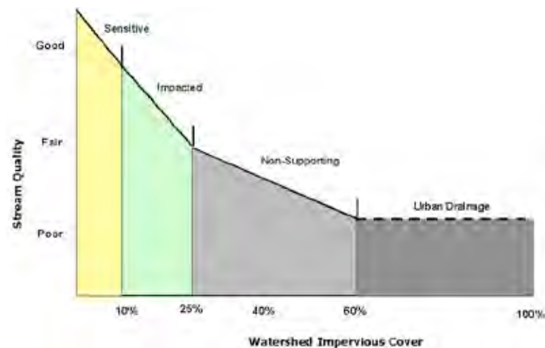
Source: Stormwater Manager's Resource Center. Relationship between impervious cover and stream quality.
